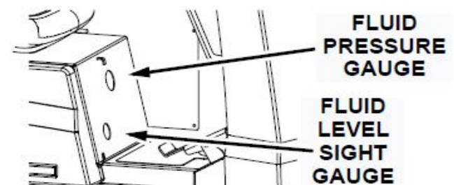
Fig. 3: Hydraulic Fluid Gauges
